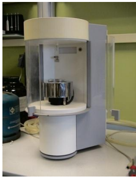
Figure A.4. Krüss K-11 tensiometer used to determine the surface and interfacial tension.
