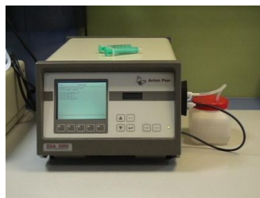
Figure A.5. Anton Paar DSA 5000 density and sound analyser.
