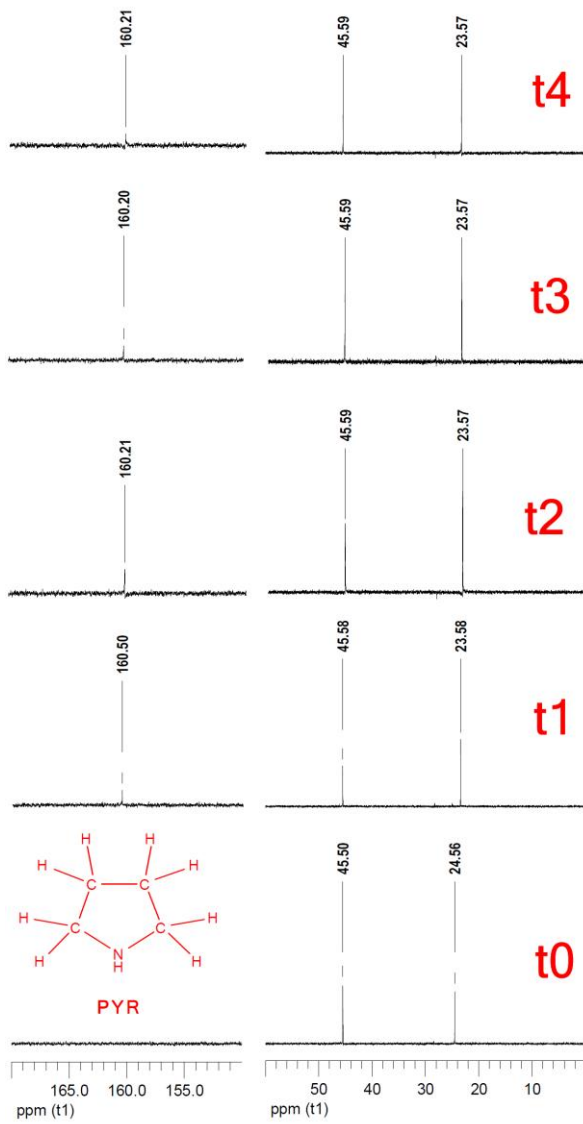
Figure 2.28. 13 C NMR spectrum corresponding to the chemical absorption of carbon dioxide in aqueous solution of pyrrolidine. C_{\text{PYR}} = 0.1 \text{ mol}\cdot\text{L}^{-1} , Q_g = 40 \text{ L}\cdot\text{h}^{-1} . (t 0 = 0 min; t 1 = 25 min; t 2 = 50 min; t 3 = 75 min; t 4 = 100 min).
