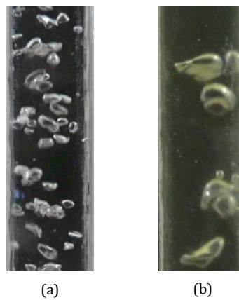
Figure 5.23. Bubbles photographs. Influence of polymer presence. (a) C_{cc} = 0 \text{ g}\cdot\text{L}^{-1} ; (b) C_{cc} = 4 \text{ g}\cdot\text{L}^{-1} . Q_g = 40 \text{ L}\cdot\text{h}^{-1} .
