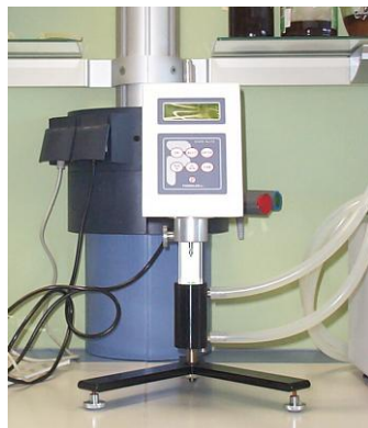
Figure A.7. Anton Paar DV-1P rotational viscosimeter
