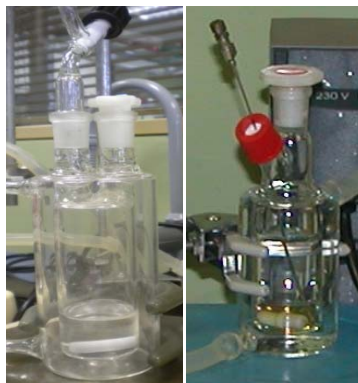
Figure 3.8. Solubility (left) and equilibrium (right) cells.
