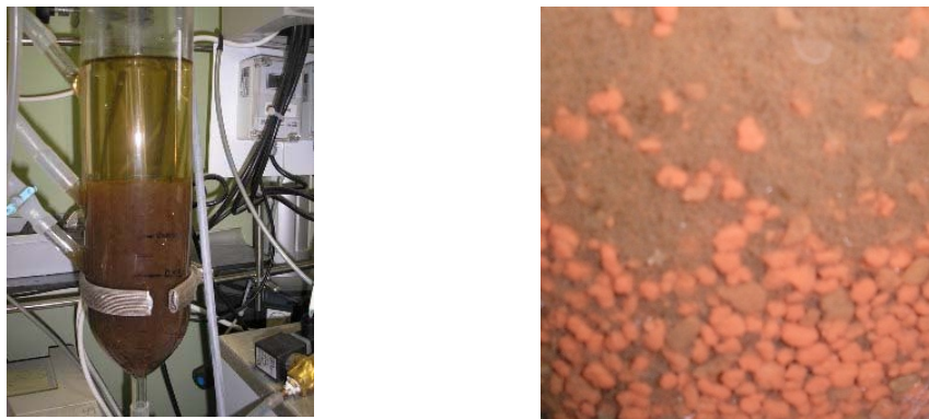
Figure 7.2. Images of the reactor and the biomass inside the reactor on day 58 of operation.
