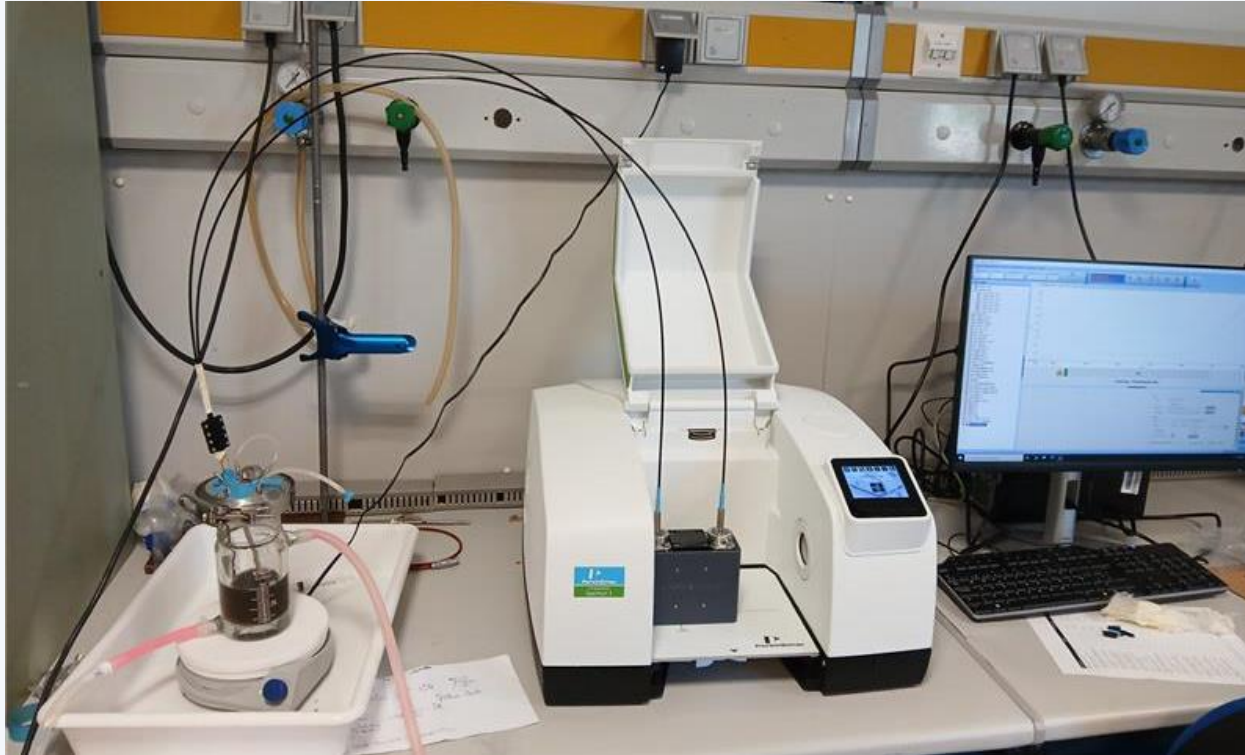
ATR diamond tip fiber probe Spectral range 600-1900 \text{cm}^{-1}
