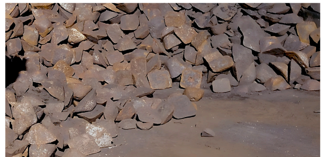
Fig. 3. Pieces of iron used to load the rotary furnace.
