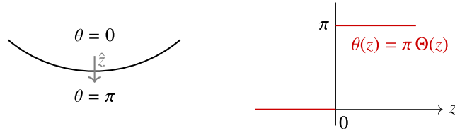
Fig. 1. Schematic illustration of a vacuum-topological insulator interface where the axion field takes values of \theta = 0 for the trivial regime and \theta = \pi for the topological insulator. We model the axion field in the boundary as \theta(z) = \pi \Theta(z) , \Theta(z) is the Heaviside step function.
