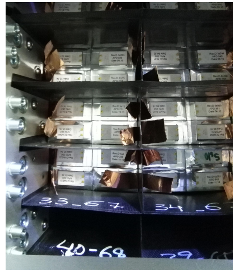
(b) Mounted crystals. Each group of four-barrel crystals fits inside a carbon fiber pocket.
