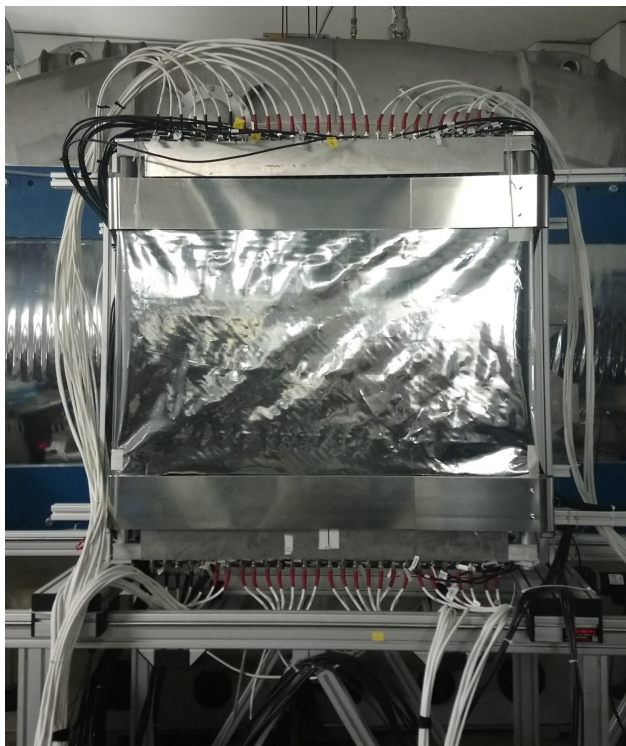
Figure 3.14: TofWall installed at the end of the beamline. The frame of the detector is shared with the MWPC3.
