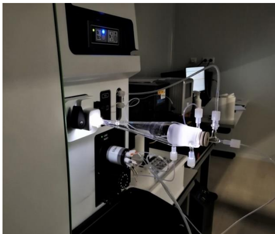
Figure 11. Single-cell-ICP-MS introduction system: innovative Asperon™ Spray chamber.
