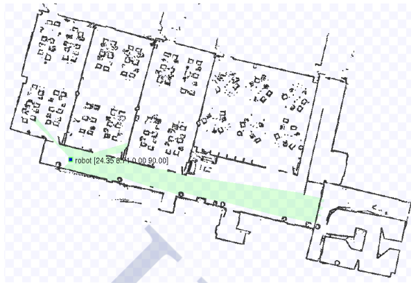
Figure 5.4: Representation of an occupancy map, a robot (blue square) and its 2D laser signature (green area).
