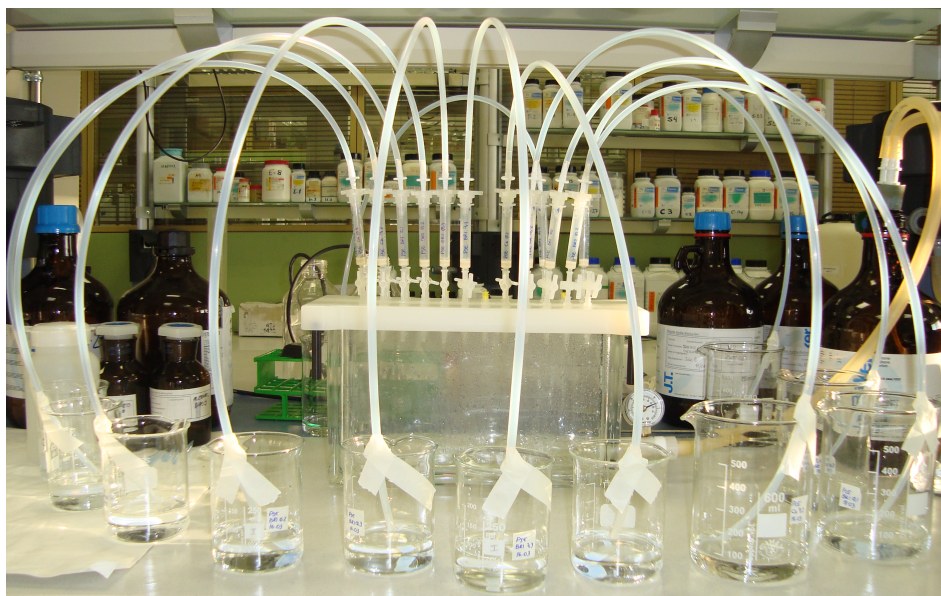
Figure 2-6. Solid phase extraction (SPE) before the GC-MS analysis
