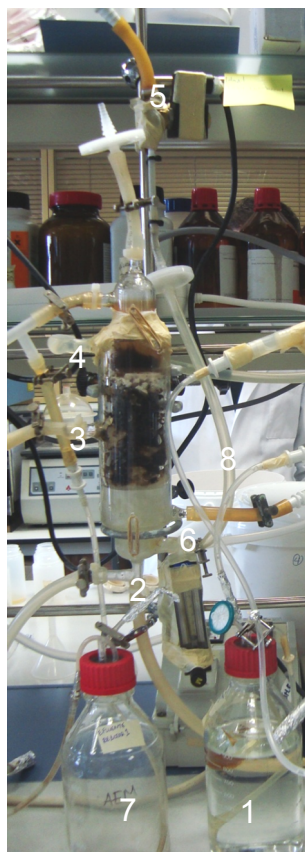
Figure 5-12. Fixed-bed reactor configuration with P. chrysosporium immobilized in polyurethane foam with oxygen pulses. Symbols: (1) feed medium bottle, (2) feed addition port, (3) reactor medium port, (4) reactor effluent port, (5) pulsing device, (6) oxygen supply port, (7) effluent bottle, (8) thermostated water.
