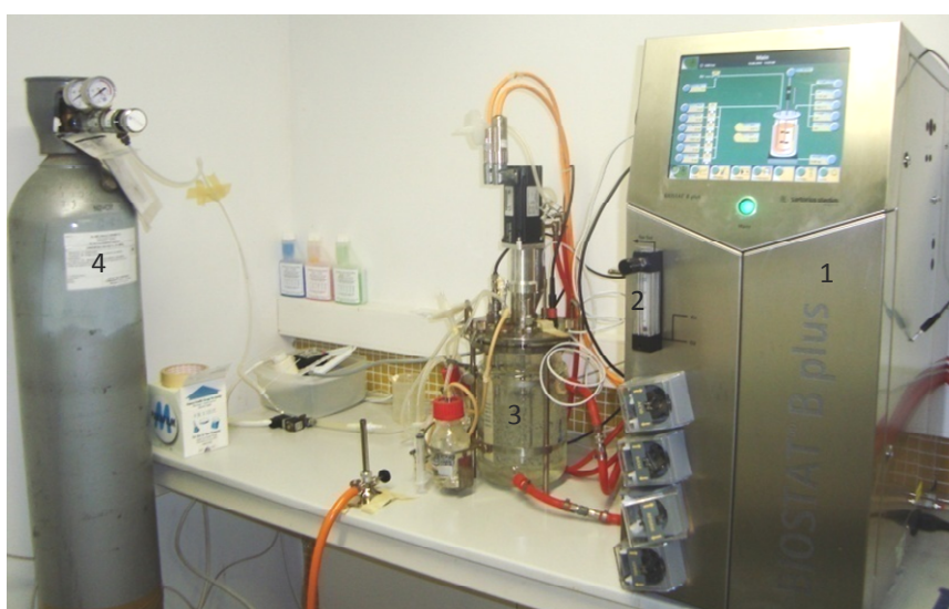
Figure 4-3. Configuration of a STR operated as fed-batch with fungal pellets. Symbols: (1) module operator service program, (2) air supply, (3) vessel with fungal pellets, (4) oxygen supply
