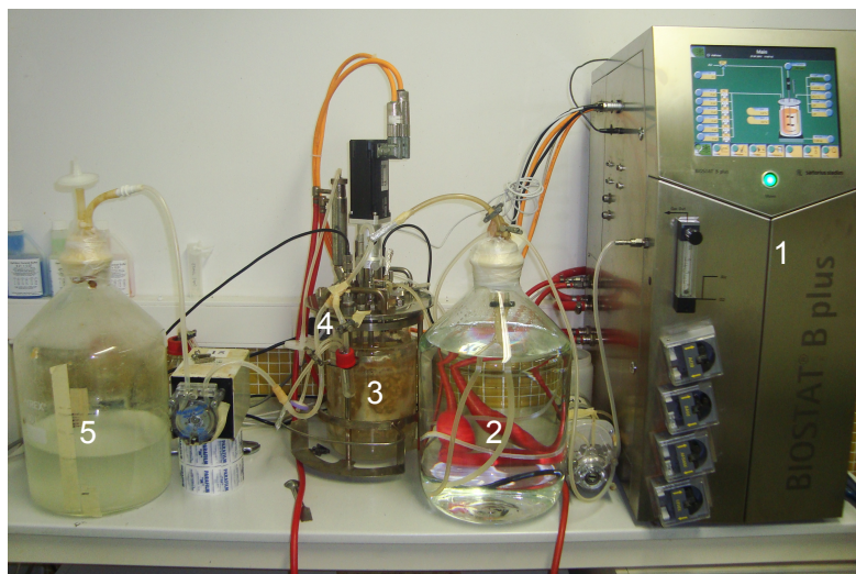
Figure 4-13. Configuration of a STR with fungal pellets during a continuous operation. Symbols: (1) module operator service program, (2) feed medium port, (3) reactor vessel filled with fungal pellets, (4) effluent sampling, (5) effluent reservoir
