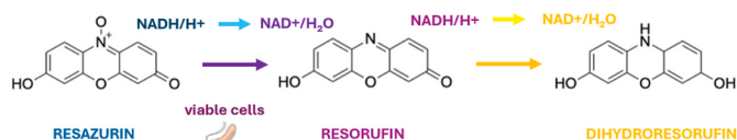
Fig. 1. Reduction of resazurin by viable cells and formation of resorufin product. Acidic environments enhance reduction of resorufin into dihydroresorufin. Resazurin, a non-fluorescent blue dye, is converted into resorufin, a pink product with high fluorescence emission. Fluorescence emission stops when resorufin is reduced into dihydroresorufin, a yellowish-white molecule.
