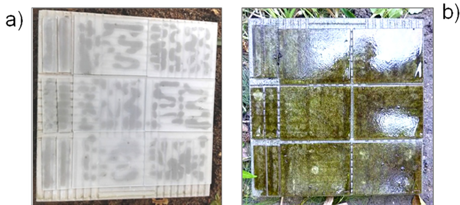
Fig. 2. Experimental setup at the Anllóns River. Artificial substrates before the biofilm colonization (a) and after 5 weeks of colonization (b), when the biofilm was translocated from the Upstream to the Downstream site.
