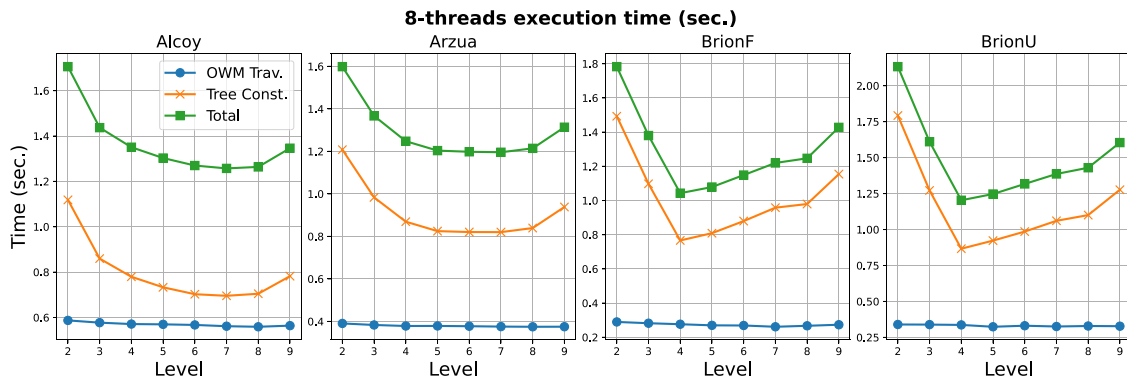
Fig. 10. Optimization O3: tree construction, OWM traversal and total times depending on lev using 8 threads.
