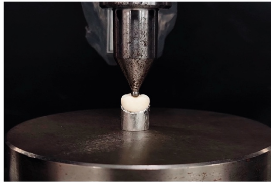
Figure 4. Loading of the specimen seated on the cobalt–chromium alloy abutment using a universal testing machine.
