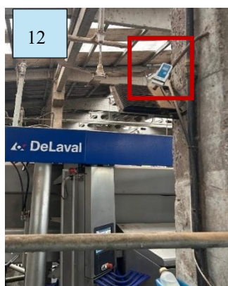
Figura 11. Dispositivo Multi-Use Compact PDF Temperature and Humidity USB Data Logger (Multicomp Pro).
