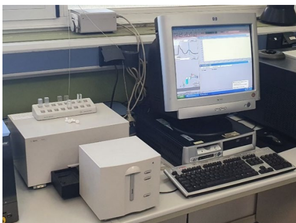
Figure 3.12. Agilent 8453 UV-visible spectrophotometer.
