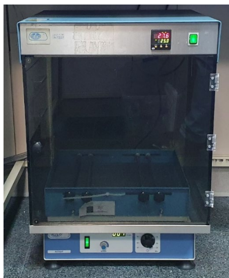
Figure 3.19. Selecta Boxcult thermostated orbital shaker.
