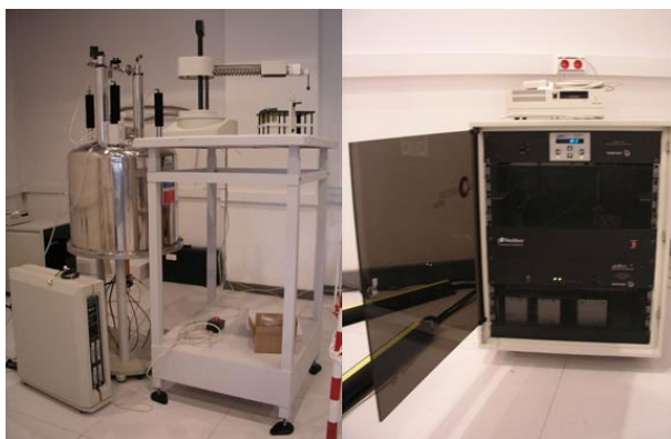
Figure 3.4. Varian Mercury 300 NMR spectrometer.
