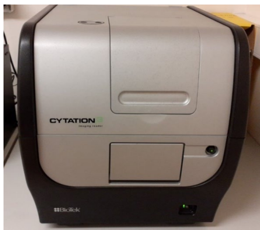
Figure 4.6. Biotek Cytation3 UV-visible spectrophotometer.
