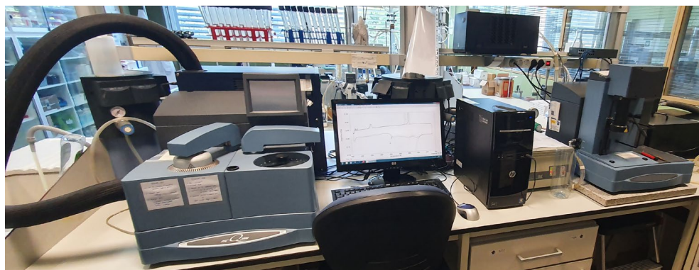
Figure 3.1. TA Instruments DSC Q2000 differential scanning calorimeter (left) and TA Instruments TGA Q500 thermogravimetric analyser.
