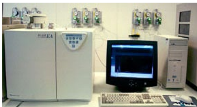
Figure 3.13. Thermo Finnigan Flash 1112 elemental analyser.
