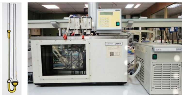
Figure 3.8. Example of micro-Ubbelohde capillary viscometer (left), and PVS1 systems installed in a Lauda D20 KP thermostat with a Lauda DLK 10 cooler attached (right).
