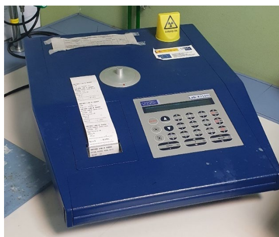
Figure 3.14. Oxford Instruments Lab-X3500S spectrometer.
