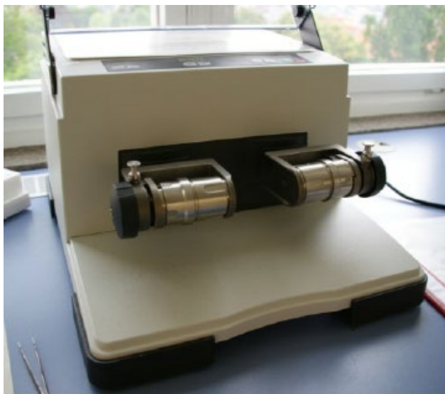
Figure 3.18. Retsch MM-2 vibration mill.
