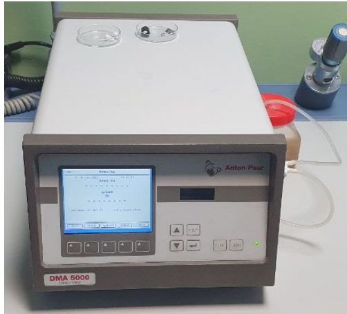
Figure 3.9. Anton Paar DMA 5000 oscillating U-tube density meter.
