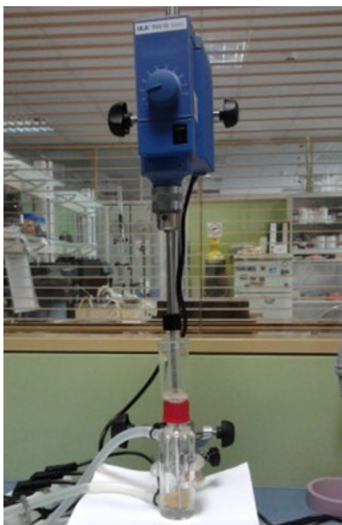
Figure 3.11. IKA RW 16 Basic overhead stirrer installed on a jacketed glass cell used for cellulose pretreatments.
