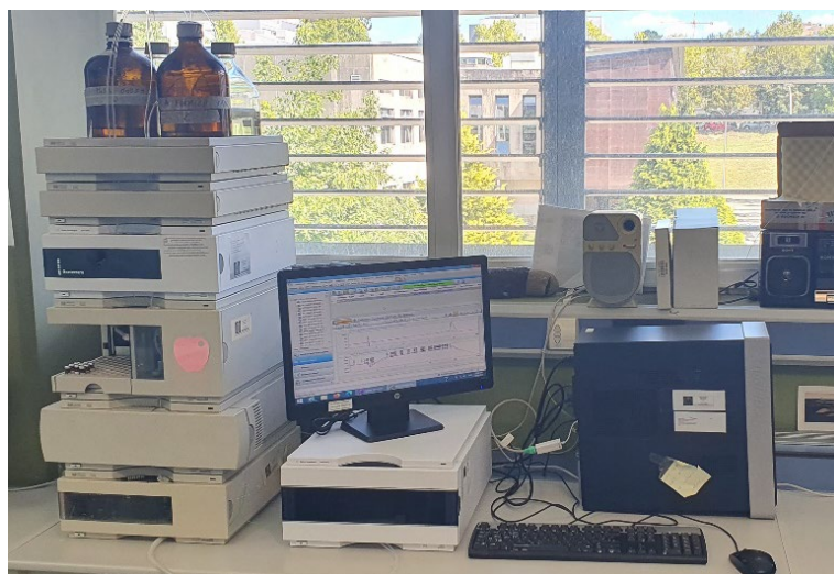
Figure 4.7. HP Series 1100 HPLC chromatograph.
