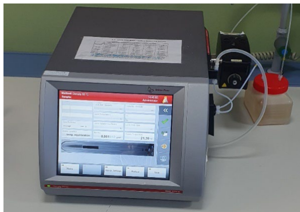
Figure 3.10. Anton Paar DMA 5000 M oscillating U-tube density meter with an attached Anton Paar LOVIS 2000 ME microviscometer module.
