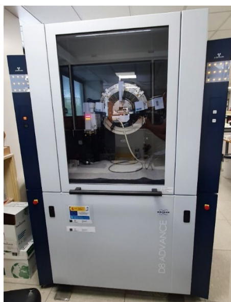
Figure 3.17. Bruker D8-Advance X-ray diffractometer.
