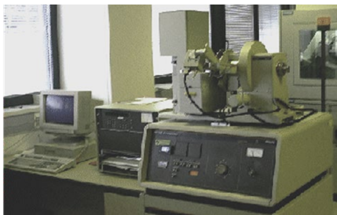
Figure 3.16. Philips X-ray diffractometer.
