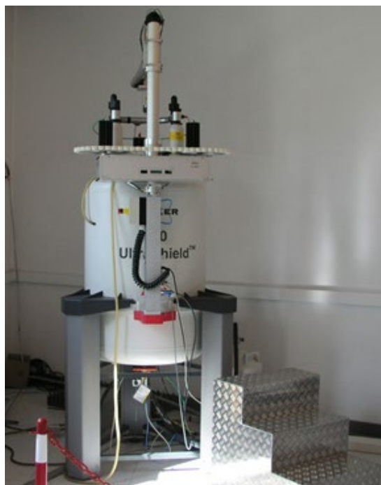
Figure 4.9. Bruker DRX-500 NMR spectrometer.
