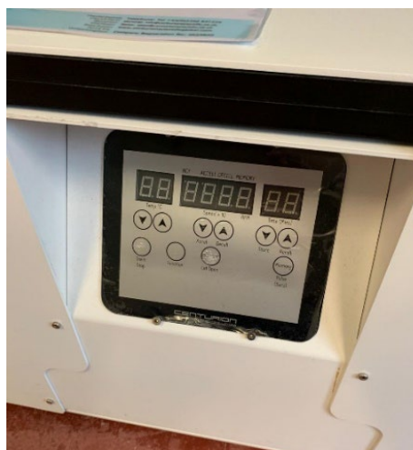
Figure 4.4. Centurion Pro-Xtra3r refrigerated centrifuge.
