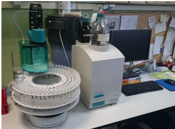
Figure 3.6. Metrohm 861 Advanced Compact IC chromatograph.
