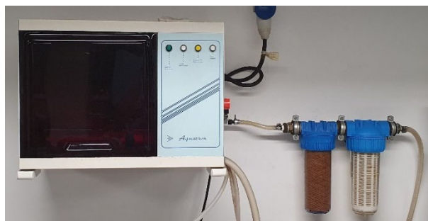
Figure 3.3. Bibby Aquatron A4000D water still for the production of bidistilled water.
