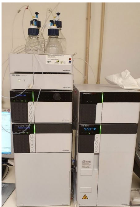
Figure 4.8. Shimadzu Nexpera X2 UHPLC chromatograph.
