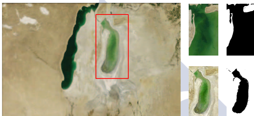
Figure 1.16: Aral sea in 2011 (left). Areal sea's region of interest in 2000 and in 2011, respectively (center). Fisher linear discriminant (right).
