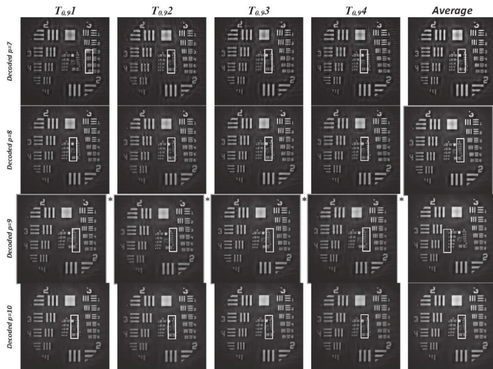
Fig. 6. Temporal sequence of restored images for r_0 = 0.9 \text{ mm} with the different JFPMs. The last column shows the restored image from the average intermediate images. White asterisks point out the best JFPM ( p value) needed for decoding. Group 5 of the USAF image is framed for further analysis.
