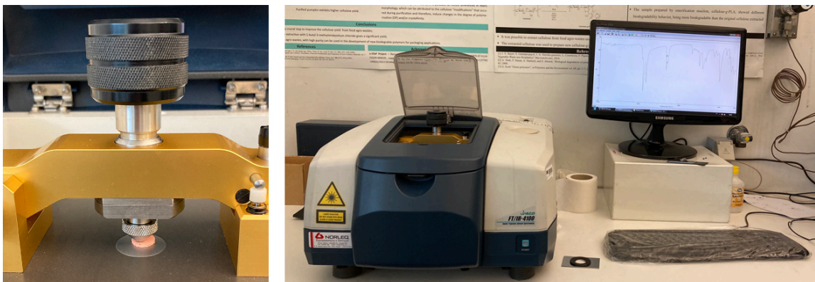
Figure 7. Fourier transform-infrared spectroscopy (FT-IR) analysis of the GP samples, using a Jasco FT/IR 4100 system (Jasco International; Hachioji, Tokyo, Japan). (Source: own elaboration)
