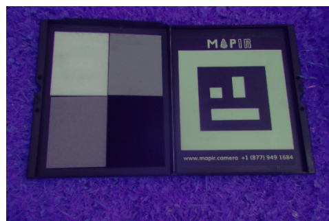
Figure 5. Calibration target V2 (MAPIR).
