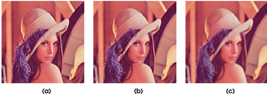
Figure 2.1: Anisotropic diffusion vs Gaussian filtering: (a) Lena image, (b) Anisotropic diffusion applied, and (c) Gaussian filtering applied.
