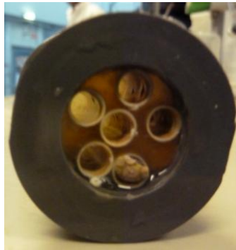
Figure 13. Membrane skid 6x (sectional view)
