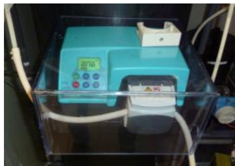
Figure 16. Feed Pump (P-402)
