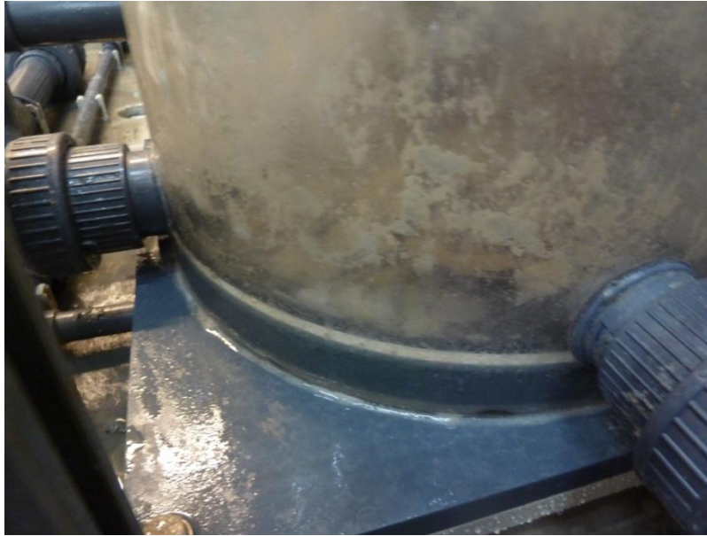
Figure 10. Inorganic precipitates fixed to the reactor walls
