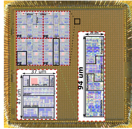
Fig. 10: HOPBAS10K microphotograph with the layout of 4 PEs and PE area breakdown.
