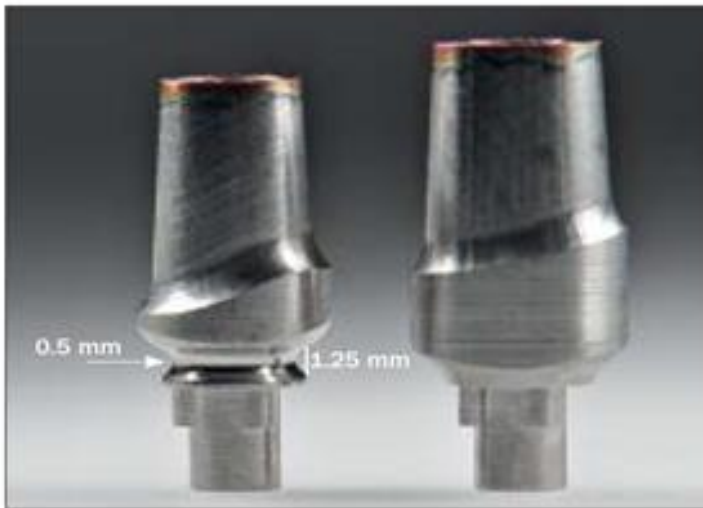
Figura 11: Pilar propuesto por Patil y cols. (Left) experimental abutment design with circumferencial groove and (right) regular abutment design (132) .
