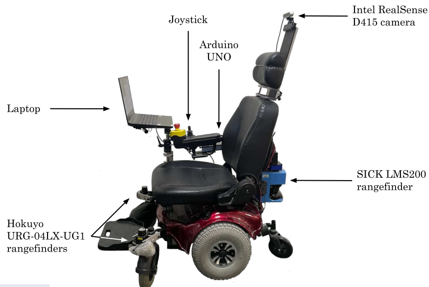
Figure 5.2: Our smart wheelchair in the configuration used for this work.
