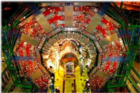
Figure 1.10 Picture of one of the five CMS DT wheels. DT chambers are inserted in the red steel structure used for support and to return the magnetic coil field.
