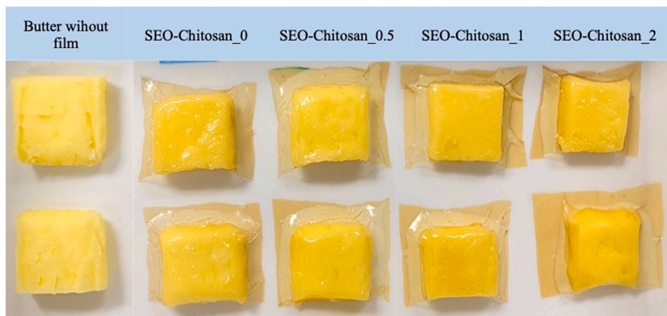
Fig. 5. Butter samples sealed in SEO-chitosan films stored at 4°C for 90 days. SEO is sandalwood essential oil.
