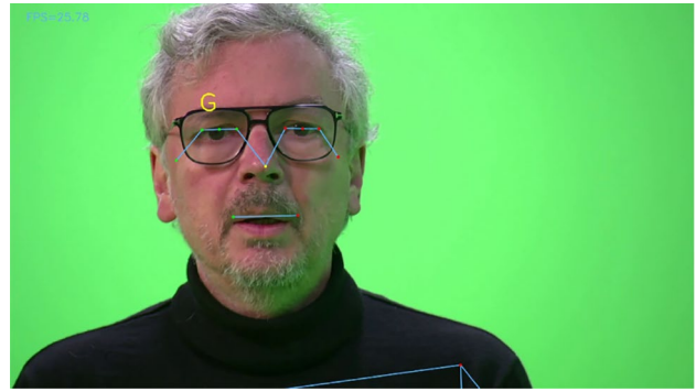
Fig. 6 Real time BlazePose-OpenVino result in short shot framing. In these cases, pose detection is not viable
