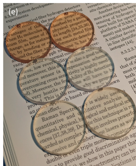
Fig. 3. Transmittance curves obtained for the resins: (a) Amber, (b) Clear, (c) Dental, (d) Flexible and Elastic. (e) Visual inspection of the transparency achieved by the discs of the three resins with both (left) and neither (right) face polished. NN: Neither face polished (solid line); NP: a face polished (dashed line); and PP: both faces polished (dotted line).
