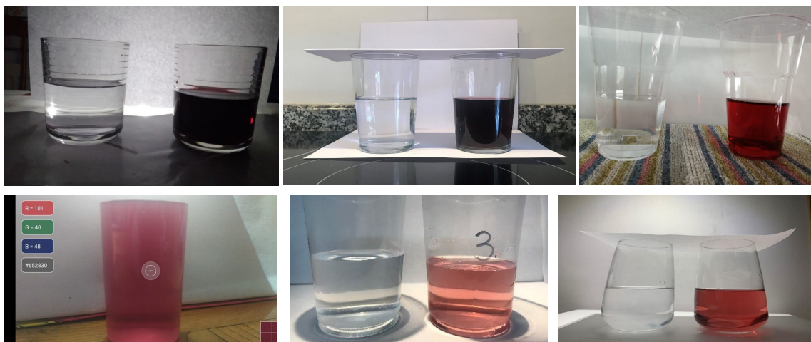
Figure 5: Examples of smartphone photos taken by the students for the absorbance measurements
