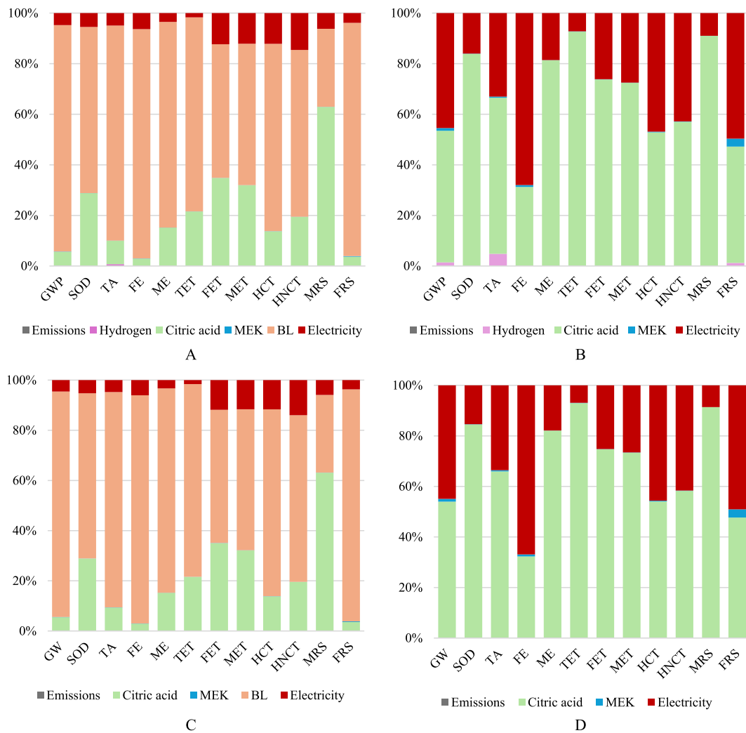
Fig. 3. Environmental profiles of worst- and best-Scenario scenario. A and B represents S2 – 600 t/d, while B considering black liquor as a zero-impact residue, C and D reports the same but for S3 – 300 t/d.
