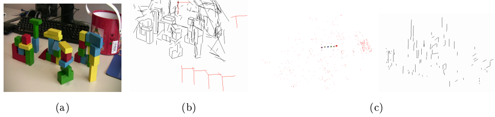
Figure 9: Qualitative comparison using the dataset Building-Blocks [22], of resolution 1440 \times 1080 . The used subset comprises the pictures \{0,2,4,6,8,10\} . a) Sample. b) Result with the proposed method, featuring 329 lines and the estimations for the six camera pose. c) On the left, the point based obtained by VisualSfM [29], featuring 3052 points and the 6 camera poses. Based on this point cloud it was generated the result obtained by Line3D++ [10] that shown on the right picture, with just 102 segments and difficult to understand.
