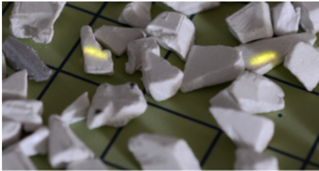
Fluorescent tracer in PVC flakes for sorting (POLYSECURE)
