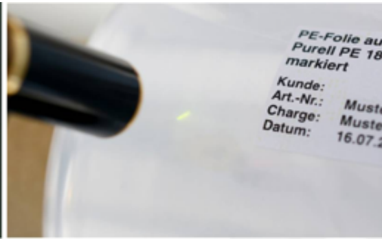
Fluorescent tracer in packaging material (POLYSECURE)
