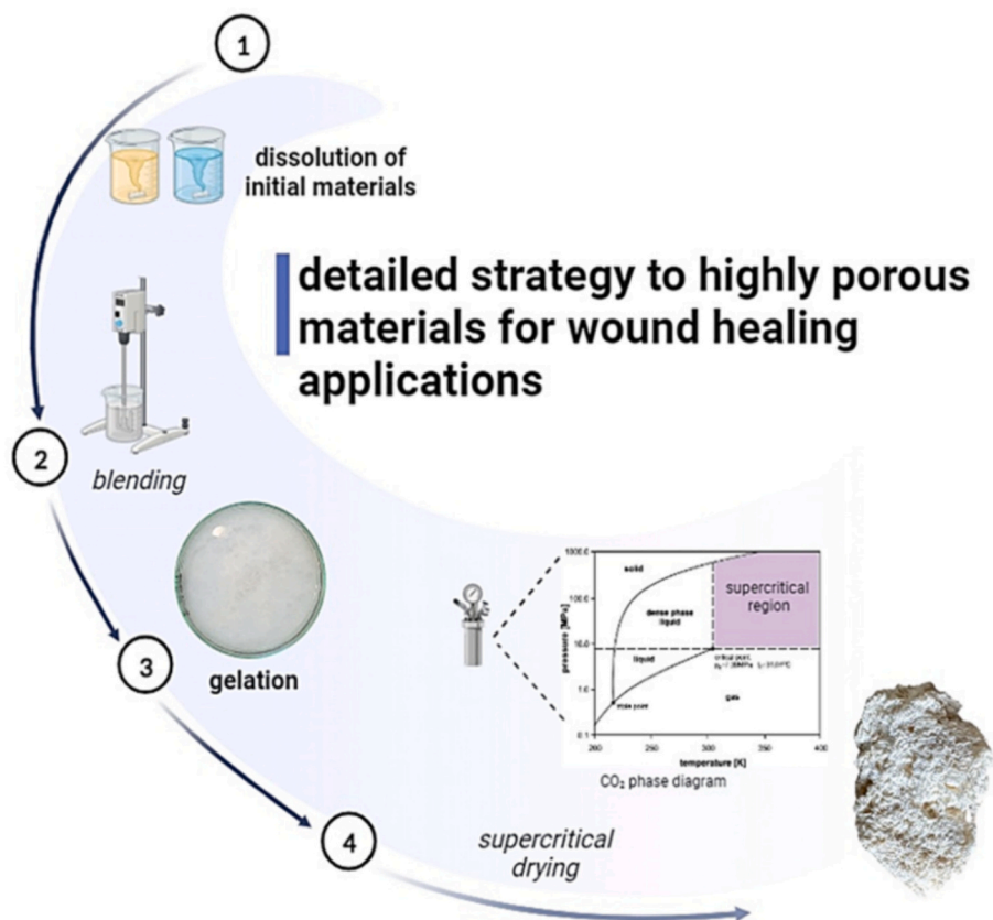
Scheme 1. Schematic of the hybrid XA/PLA-CSD aerogel synthesis process.
