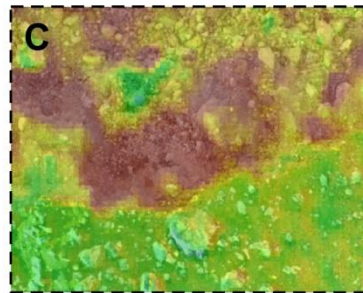
Figure 6. DEM of difference showing changes in the surface elevation of the flow between 2016 and 2018. A, B, and C provide more detailed information from three sample areas, with summary statistics illustrated in the accompany bar graph.
