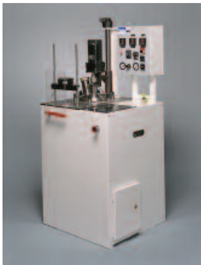
Figure 1. A semi-automatic low-pressure molding machine (Peltsman LPIM Machine MIGL-33).
