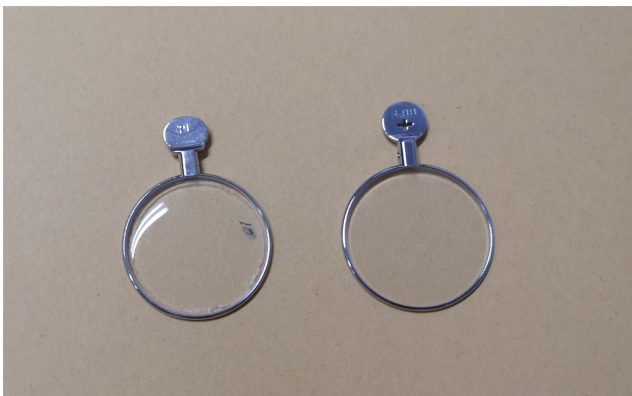
FIGURE 2 Example of the lenses used. Plano trial lens with the auto-adherent lens (left), and conventional trial lens (right).
