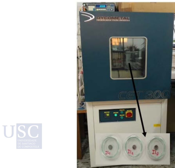
Fig. 2.16. Temperature chamber and pictures of three samples placed in Petri dishes
