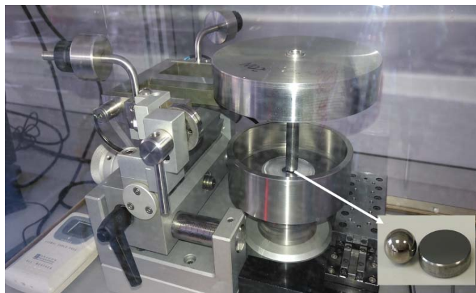
Fig. 2.12. CSM Standard tribometer with ball-on-disc configuration
