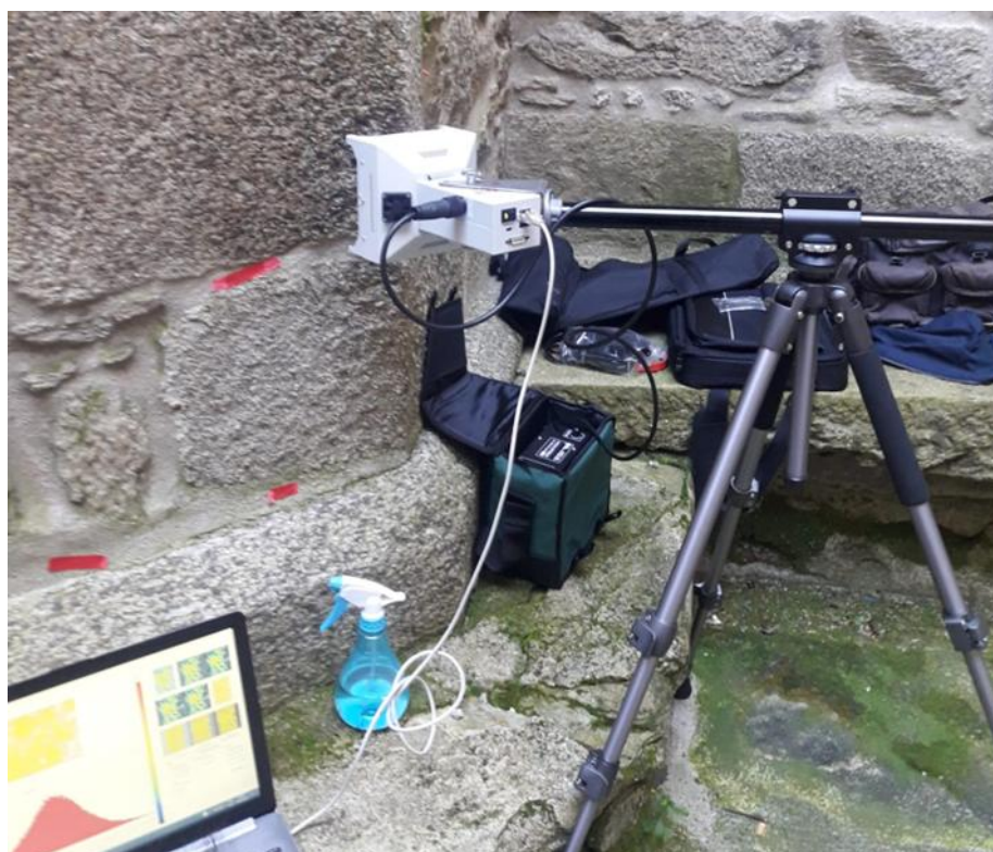
Figure 9. Use of the imaging PAM fluorometer over a granite ashlar in the inner courtyard of Pazo de Raxoi . Image by P. Sanmartín.
