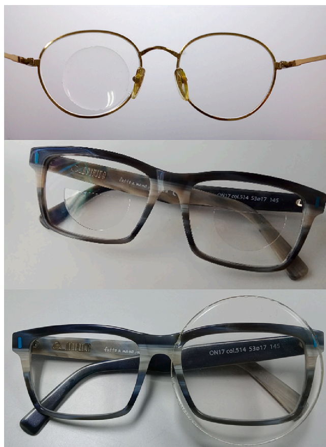
Fig. 6. Picture of spectacles with: PDMS lens (top); Hydrotac lenses (center), adhered to ophthalmic lenses; and full-frame PDMS lens (bottom).
