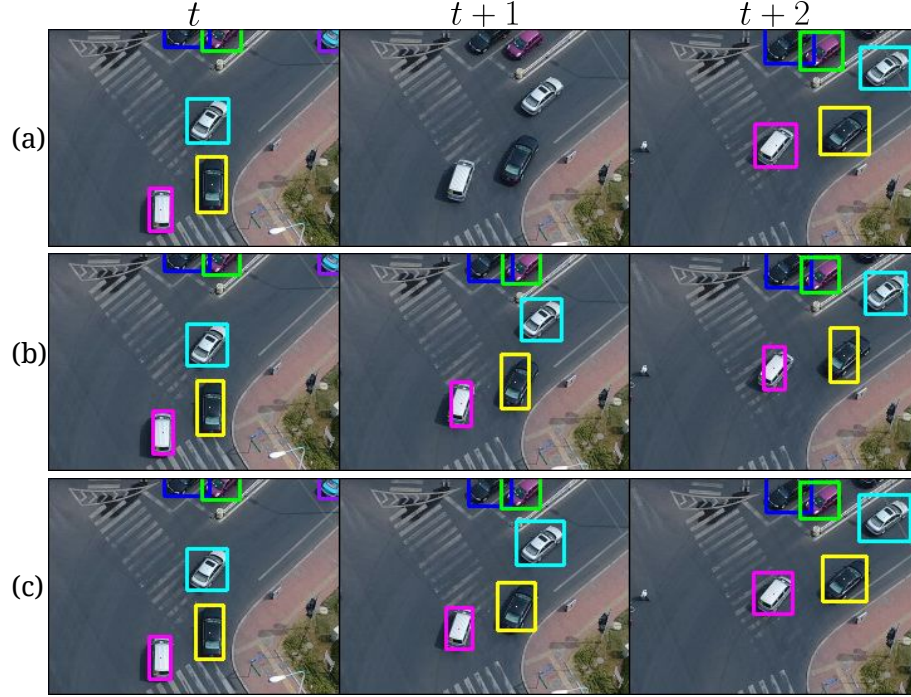
Figure 3.1: Comparison of (a) a multi-object tracking system lacking motion estimation between detections, (b) SiamMT [145], and (c) our proposal (SiamMOTION). Notice how (a) is unable to handle all frames and (b) does not detect changes in the aspect ratio of the objects.
