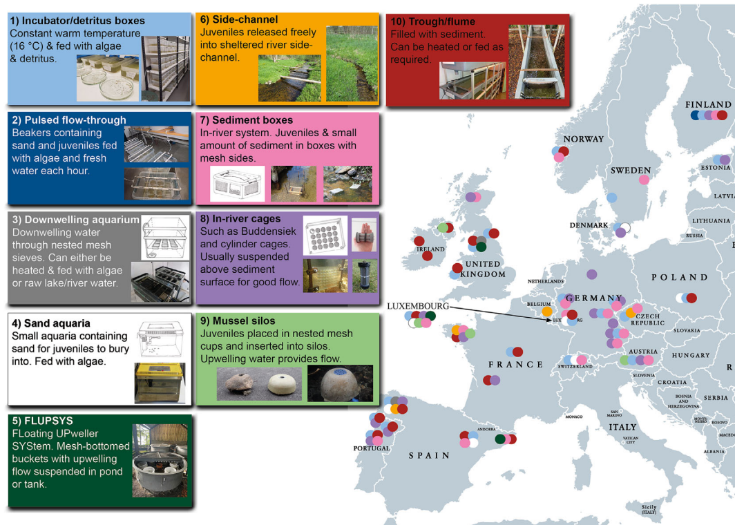
FIGURE 1 Captive breeding methods used for freshwater mussels throughout Europe. Coloured dots on the map refer to the different techniques described in the note boxes. Boxes 1 and 2 describe high-intensity methods, requiring maintenance at least once per week; boxes 3–5 describe medium-intensity methods, requiring maintenance at least once per fortnight; and boxes 6–10 describe low-intensity methods, requiring maintenance approximately monthly, or as needed
