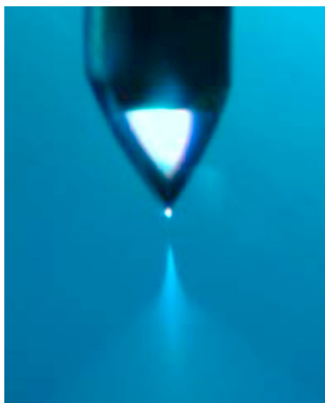
Figure 1. Electro-spray in cone-jet mode with aerosol formation. Reprinted with permission from ref 13. © 2018 Elsevier.
