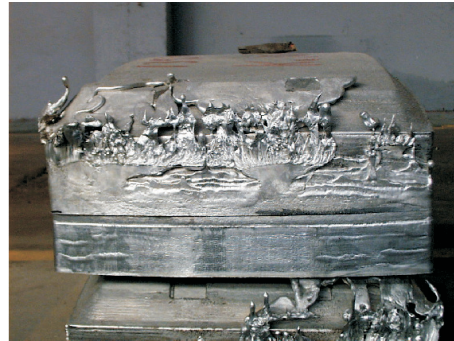
Figure 13.2: Butt curl deformation. Imaged provided by ALCOA-INESPAL S.A.
