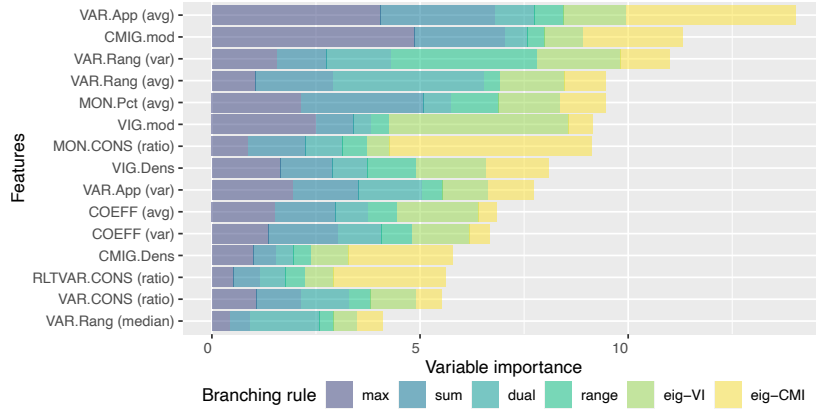
FIGURE 5.5. Stacked bar graphs represent, for each branching rule, variable importance score of the features obtained using Q-RF.
