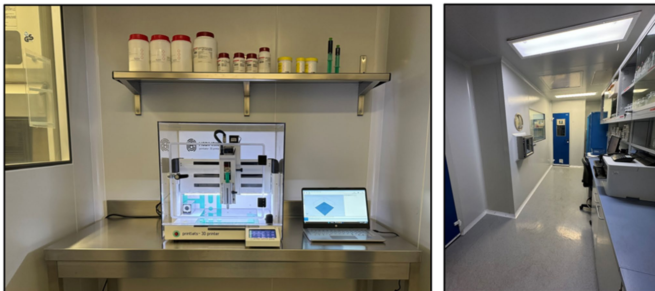
Fig. 5 The left image depicts the pharmaceutical 3D printer M3DIMAKER™ in the Good Manufacturing Practice manufacturing room within the hospital pharmacy. The right image shows another section of the manufacturing room, featuring the entrance door to the printer room
