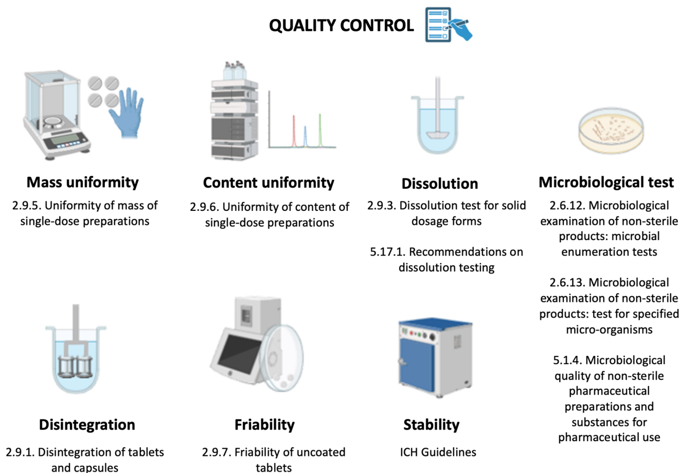
Fig. 3 Main quality control tests applicable to solid printlets according to Ph. Eur
