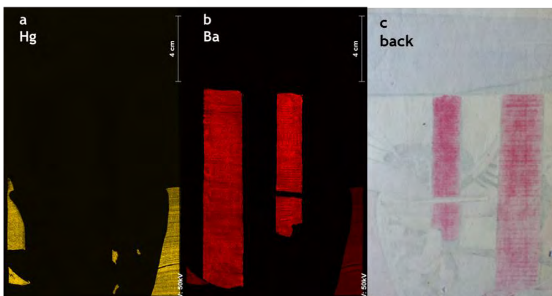
Figure 3.46: MA-XRF elemental mapping of vermilion (Hg) (a), and lake-baring organometallic mixture of azo \beta -naphthols precipitated on barium sulfide (Ba) (b); back of panel n°2 (c).
