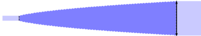
Figure 4.1: Adiabatic taper geometry [139], in this case joining a thin waveguide together with a wider one. This very shape is used also to couple light in and out of the MZIs. The shape of the curve is parabolic.
