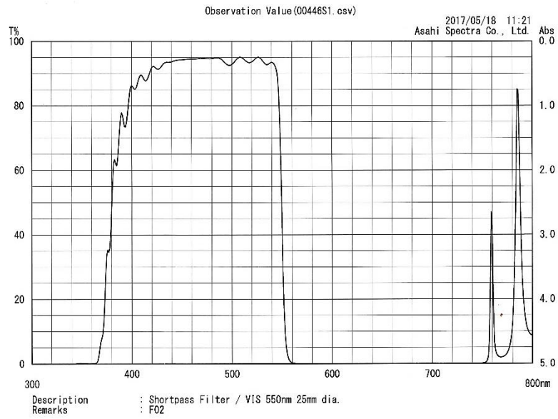
Image 1. Abs and T% spectrum of the short pass filter (VIS 550nm 25 dia.).
