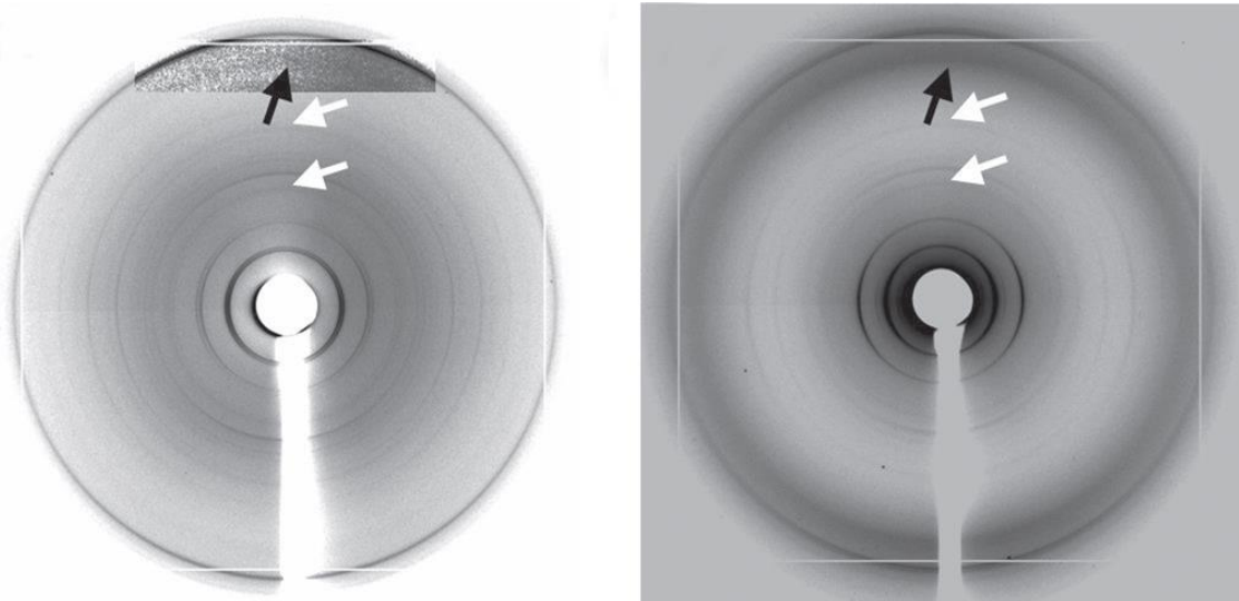
Fig 1.16. Fiber diffraction patterns from PTA-precipitated MoPrP amyloids. Black arrows indicate cross-meridional diffraction at close to 4.8 Å resolution. White arrows indicate second and third orders of meridional 19.2 Å diffraction. (A) MoPrP 27-30(RML). Inset uses a different color table to show the weak, broad 4.8 Å diffraction. (B) The synthetic prion strain, MoSP1, derived from recPrP (89-230) amyloid, passaged twice through Tg9949 mice and purified as in A. (Open access).
